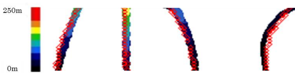
Figure 4 – Clustering of 7 control point trajectories. Four samples of real trajectory (red circles) and the corresponding category found by our clustering process. Each cluster is defined as color coded superposition of trajectories, where color is associated with future travelled distance (see legend on the left side)
